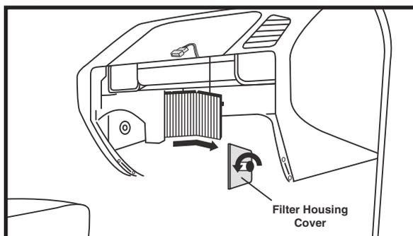
17. Turn wheel on filter housing cover 90° counter clockwise.
