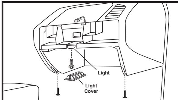
9. Remove screws on either side of glove compartment opening.
