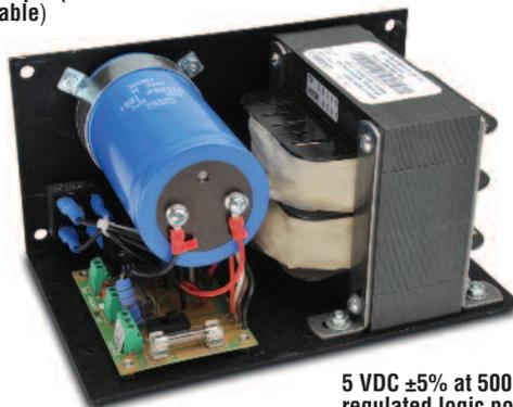
5 VDC ±5% at 500 mA regulated logic power
