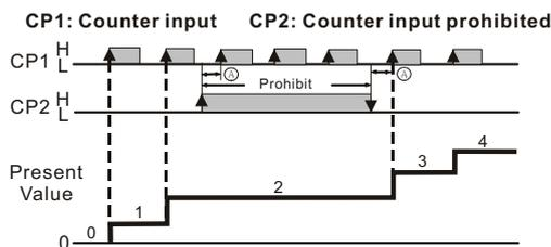
Note: (A) has to be larger than width of min. Input signal
