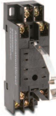
Din-rail mounting, DPDT, for use with QM2 series relays
