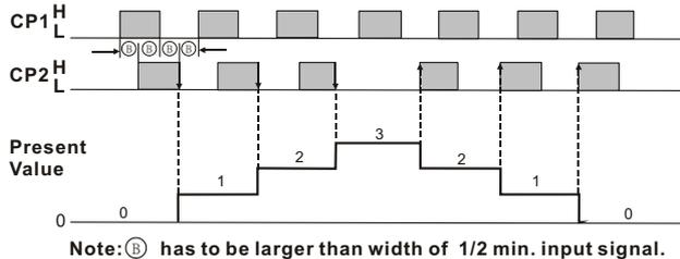
Note: (B) has to be larger than width of 1/2 min. input signal.
