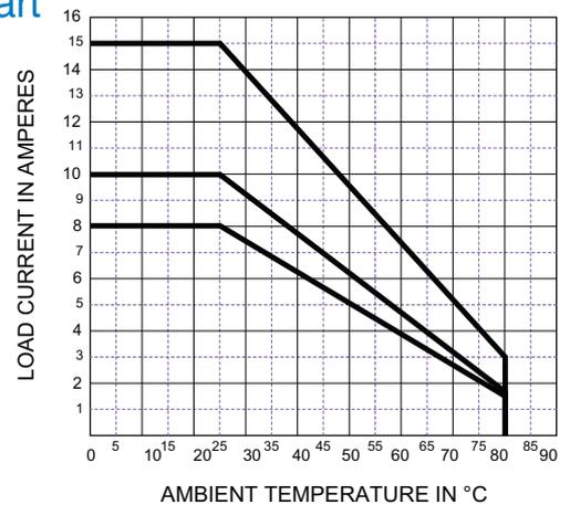
**Note:** A minimum spacing of 17.5 mm (0.7 in) between adjacent 861 relays is required in order to achieve the maximum ratings. A 0mm spacing will result in a 50% reduction in the de-rating.
