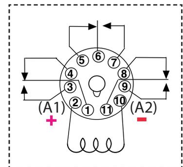
*Note: Contacts and coil shown are internal to the relay*
