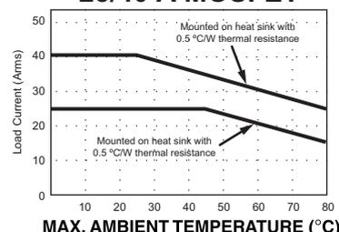
Note: Charts are based on using a thermal transfer medium such as the included thermal pad
