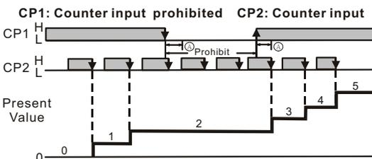
Note: (A) has to be larger than width of min. Input signal
