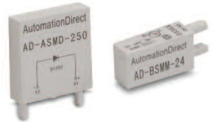
When inductive load devices (motors, motor starters, interposing relays, solenoids, valves, etc.) are controlled with relay contacts, it is recommended that a surge suppression device be connected directly across the coil of the field device. If the inductive device has plug-type connectors, the suppression device can be installed on the terminal block of the relay output.
