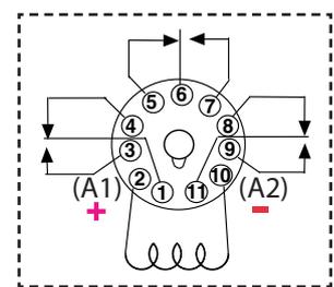
Note: Contacts and coil shown are internal to the relay
