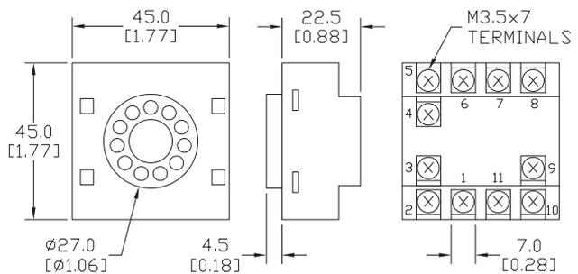
**Cutout for panel mounting TP48SB and TP411SBA sockets using PANEL-16 mounting clips**
