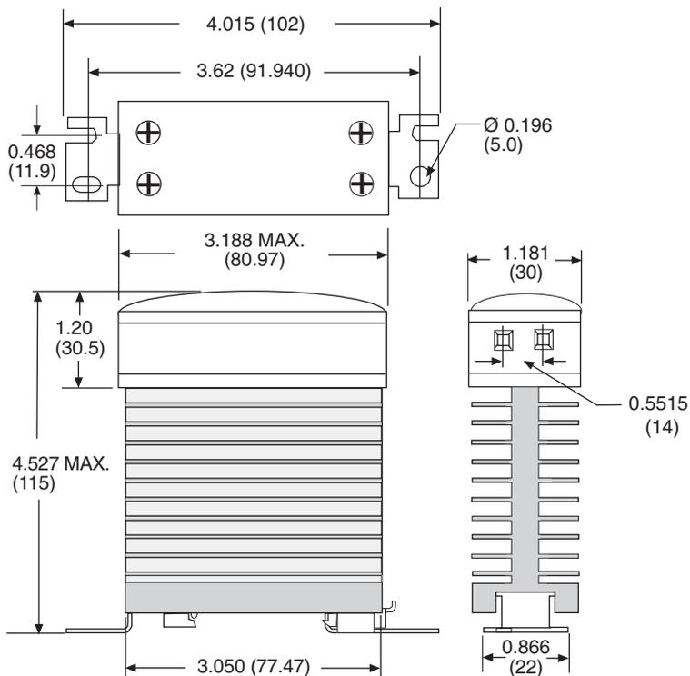
Note: Recommended spacing between multiple SSRs is 0.75 inch.
