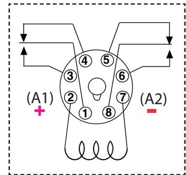
*Note: Contacts and coil shown are internal to the relay*
