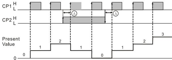
Note: (A) has to be larger than width of min. input signal.
