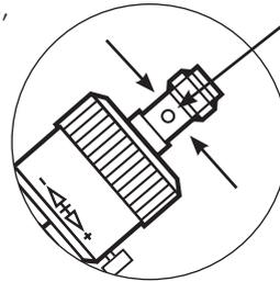
There are 4 LEDs (one on each side) on the top connector for easy visibility regardless of installation orientation.
