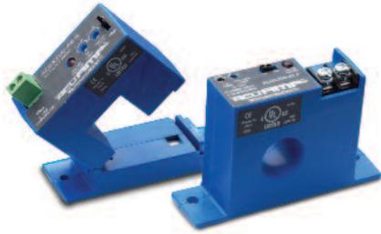
The ACSX series high-performance current-operated switch has a field-adjustable time delay feature that minimizes nuisance trips during start-up and operation. These switches are designed for motor status applications where setpoint accuracy and repeatability are critical and offer a linear setpoint characteristic and constant hysteresis.
