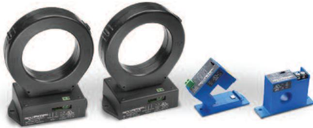
ACT current transducers combine a current transformer and signal conditioner into a single package. The ACT series has jumper-selectable current input ranges and industry standard 4-20 mA or 0-10 VDC outputs. The ACT series is designed for application on 'linear' or sinusoidal AC loads and is compatible with most PLCs, data loggers and SCADA systems. Full-scale input ranges are user-selectable from 2A to 2000A. This series is available in split-core or fixed-core models.
