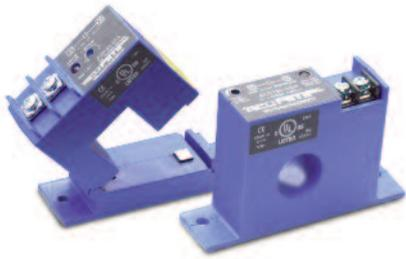
ACS150 Series current operated switches combine a current transformer, signal conditioner and limit alarm into a single package for use in monitoring or proof of operation applications. Offering an adjustable setpoint range of 1 to 150 amps and universal, solid-state outputs, the self-powered ACS150 can be tailored to provide accurate and dependable digital indication of over-current conditions across a broad range of applications. The ACS150 is available in fixed-core and split-core models.
