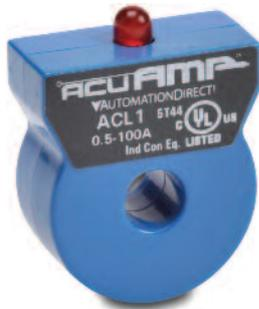
The ACL1 Current Indicator is a small, inexpensive, simple LED ring which slides over a conductor to give a flashing indication of current flow. This unit is ideal for use in control panels, or wherever you need to substantiate current flow. The ACL1 current indicator is a cost-effective way to detect live conductors and see current flow to fans, heaters, pumps, lighting or other powered devices.
