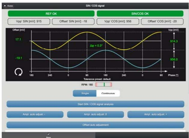
Display of the SIN/COS signals for the signal analysis information on the tooth-to-tooth values and indication of the average values over one turn
