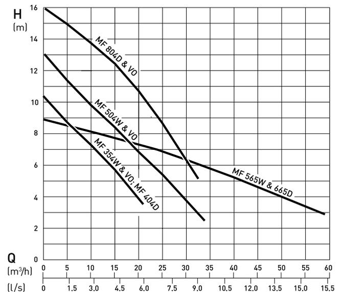
H = Total Head; Q = Discharge Volume. Curves to ISO 9906 (60 Hz available on request) N.B. please use the ABSEL program to validate pump selection.
