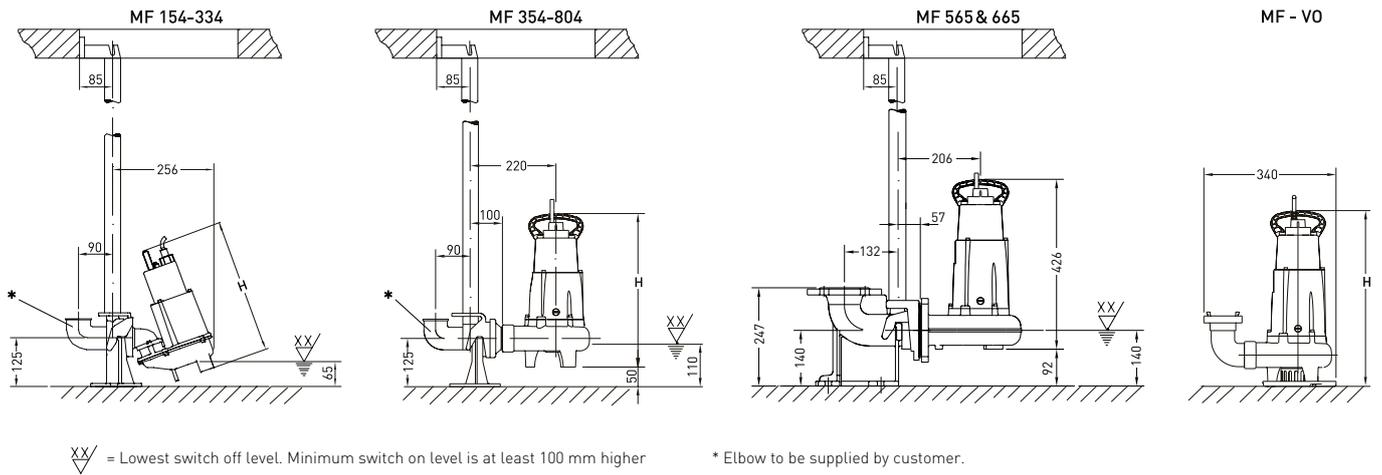
XX = Lowest switch off level. Minimum switch on level is at least 100 mm higher
